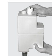
4. Turns on water box lid, fill well full water tank, and tightens lid, installs in the machine according to the original order.
